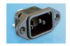
The Corcom SR Series includes a full line of popular AC receptacles. These male and female power line connectors include snap-in and flange mounted models. Now available in 20 Amp versions with flange mount and snap-in configurations. These AC receptacles feature a standard IEC60320-1 inlet for power cords and quick-disconnect terminals for load side connection.
